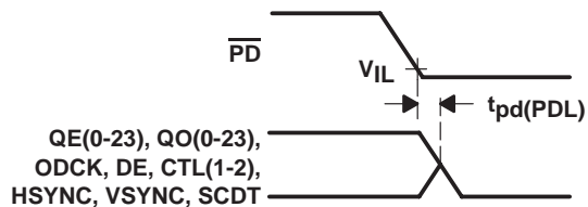
Figure 7. Delay From \overline{PD} Low to Hi-Z Outputs
